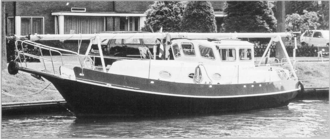
The pilothouse on the 28-foot Spray K*I*S*S has reverse-sloping windows up forward, and while they may not be to everyone's taste, they do have many advantages, two of which are lack of glare and reflection and absence of moisture in light rain conditions.
