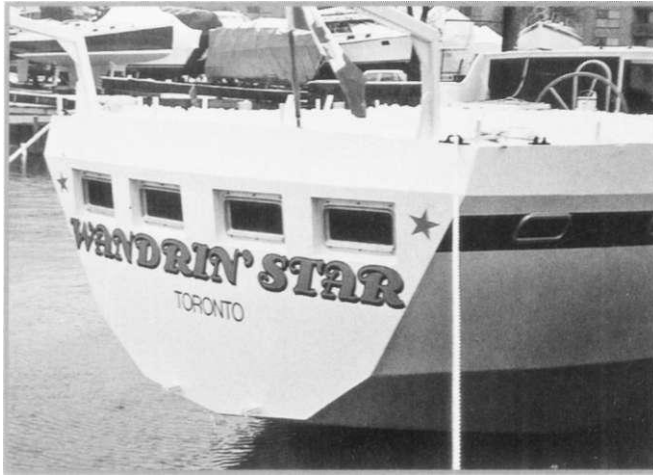
Recessed ports and windows always add a professional finish to any metal hull; these are fitted to a Roberts 64 built in Canada.
