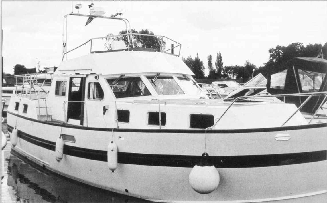
The long-lasting paint job on this early version of the Waverunner 34 proves the benefits of using pre-prime-coated steel.
