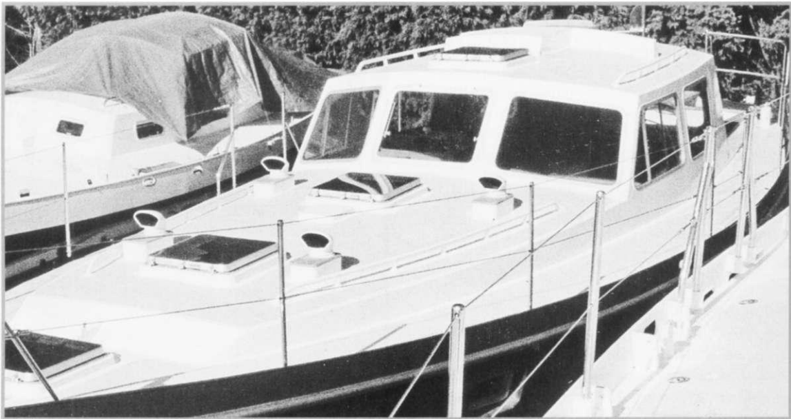
The low cabin on this Roberts 39 will receive adequate light and ventilation from the opening hatches and dorade vents.
