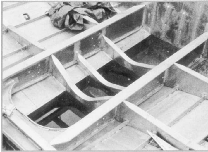
These engine beds embody many of the features described in the text
