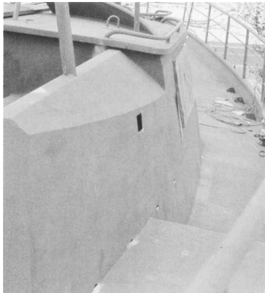
The beveled cockpit coaming adds to the attractive appearance of this Roberts 53 built in Canada by A. Skodt.
