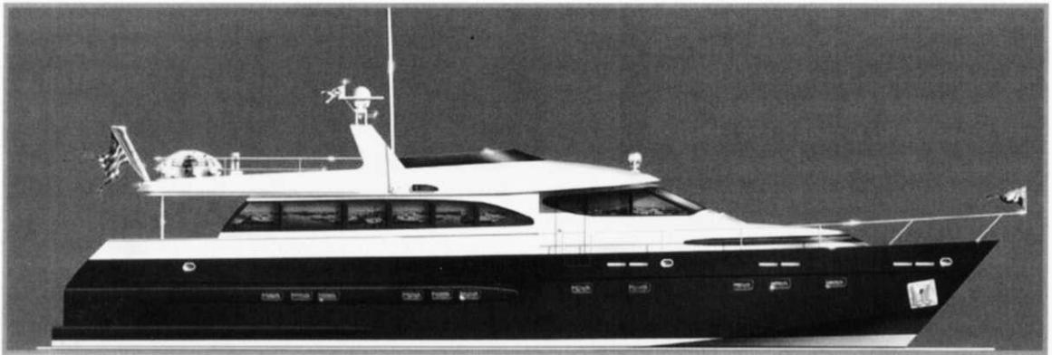
The Euro 2300 version is a semidisplacement motor yacht (12-15 knots) and the Euro 2400 is a planing hull configuration (16-30 knots). The underwater shape of the hull together with the horsepower of the engines govern the performance and cruising speed that you can expect from this and other similar Euro Series Motor Yachts.
