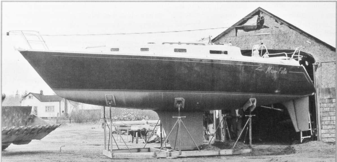
This Roberts 342, built in Europe, is a fine example of what you can achieve using the radius-chine technique to build in either steel or aluminum.
