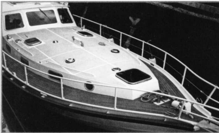
This steel Spray 40 shows several attractive and sensible features, including substantial pipe guardrails (stainless would have been nice) and a nicely laid teak deck. Note the wide covering board around the edge, a sturdy pair of stainless steel bollards on the foredeck, a timber rubbing strip "stood off" the hull, a pair of stainless steel bow fairleads, and a well laid out fore-cabin top.
